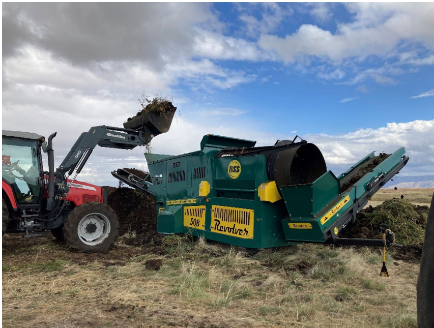
Manure screener at Asotin Conservation District, photo courtesy of Alison Halpern, SCC
